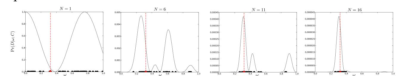
This figure demonstrates the flow of probability mass and particles as the algorithm processes data. The red dot and line represent the randomly selected "true" model while the black dots are the SMC particles (the weights are uniform here).
