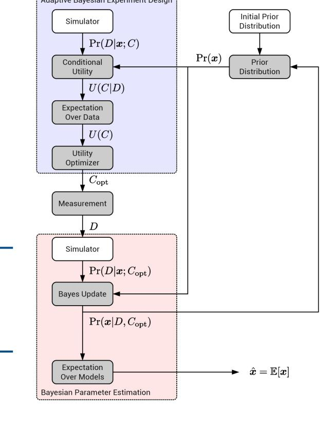
Expectation values can now be computed as finite sums, and the Bayes update step can be computed with one calculation per SMC particle.
